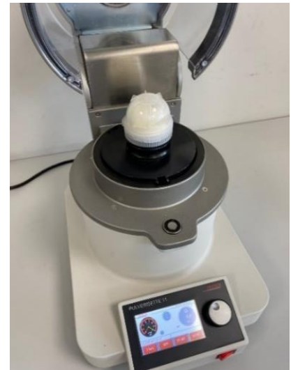
Sample in 40 ml single-use grinding vessel in our Knife Mill PULVERISETTE 11
